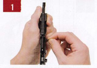
Insert charging handle with the flat end toward the barrel.
