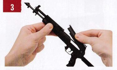
Slide on dust cover ensuring rear hooks attach and front holes align.
