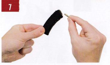
Load dummy rounds into mag. Insert mag into mag well until it clicks into place.
