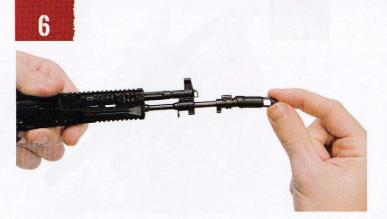
Slide muzzle break on with longer portion on the bottom of barrel. Rotate approx  $\frac{1}{2}$  turn to lock muzzle into place. Note: Muzzle break will loosen if turned more than approx  $\frac{1}{2}$ .
