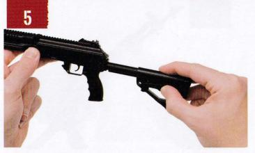
Depress lever to slide stock over buffer tube.
