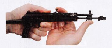
Insert dust cover pin and rotate clockwise until it latches on handguard.
