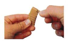
Load non-firing round (I) into magazine (H). Slide magazine into receiver until it clicks into place.
