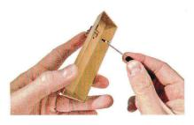
Attach mount piece (G) to display stand (F) using screw provided. Screw into place by flipping over stand. Insert screw into small hole.
