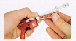
Place top (A) and bottom (B) hand-guards on barrel by pushing against spring, locking into place. Narrow (A) hand-guard on top.
