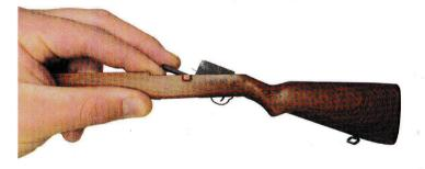
Place trigger housing group (A) in lower receiver (B). Housing group has tabs on both ends to hold it in place.
