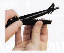
Place top (A) and bottom (B) handguards on barrel by pushing against spring, locking into place. Handguards narrow toward end of barrel.
