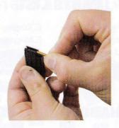
Load non-firing round (G) into magazine (F). Slide magazine into receiver until it clicks into place.
