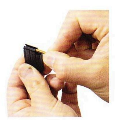
Load non-firing rounds (G) into magazine (F). Slide magazine into receiver.
