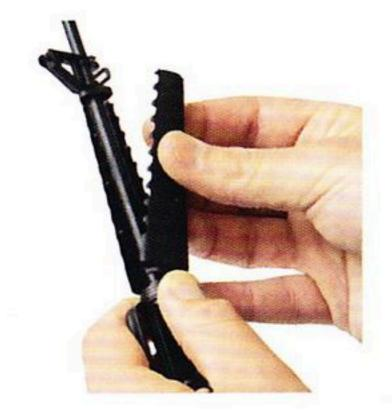
Place top (A) and bottom (B) handguards on barrel by pushing against spring, locking into place. Handguards narrow toward end of barrel.
