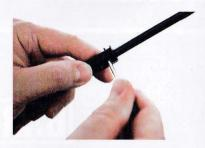
Screw barrel (C) and receiver (A) together with medium screw into hole below front sight.
