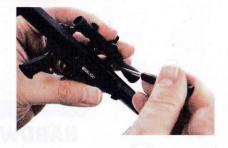
Place scope onto receiver, tighten with screwdriver.
