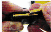
6 Load non-firing rounds (G) into magazine (F).
