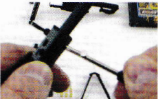
2 Screw barrel (C) and receiver (A) together with medium screw into hole below front sight.
