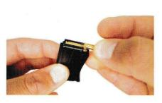
Insert 3 dummy rounds (I) into magazine (H).
