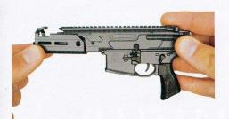
Slide handguard (A) over receiver (C) and screw into place with 2 screws.
