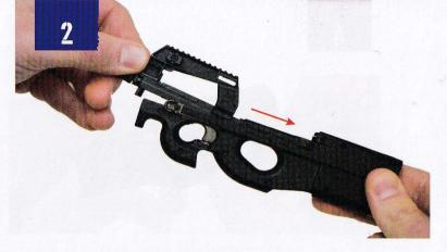
Slide upper receiver onto lower receiver.
