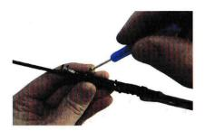
Push receiver (G) into barrel (D), insert the long screw where the holes align on top of the barrel.
