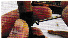
4 Slide barrel (A) onto upper receiver (B). Screw into place using one of the included screws.
