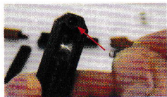
2 Place spring and retaining pin into back of upper receiver (B), inserting spring first
