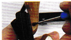
5 Screw stock (E) onto lower receiver (C).
